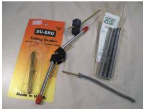
Du-Bro tool bends standard 1/8-inch-diameter tubing and includes four 3-inch tube sections. Blue Harry Higley tool works on 1/16- and 1/8-inch sizes. K&S system works on all sizes from 1/16 to 3/16 inch. All prevent kinks caused by hand bending.
