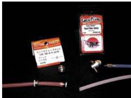
Whitish silicone fuel line is best used inside tanks. Pink Prather Products, blue Aero
