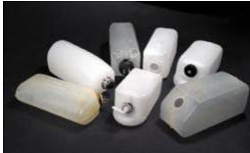
L-R: Narrow tank used vertically, flat-bottom tank for use over retract nose gear, high-pressure tank for pressurized fuel systems, standard sport square shape, square tank with "bumper" to protect fuel lines, popular space-saving "slant" tank. Center bumper tank comes with fittings installed.
